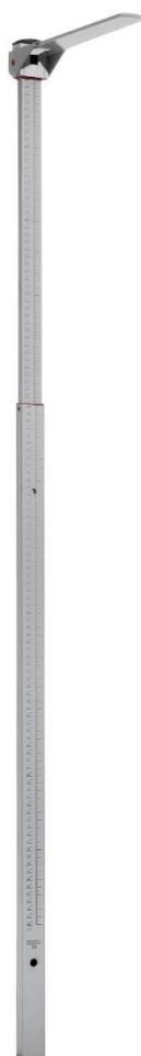
Telescopic height measure for mounting at ADE electronic column scales as well as mountable at any wall. With foldable safety head piece. The reading is practically done at eye level. Accurate to 1 mm with a measuring range of 600 – 2100 mm.
